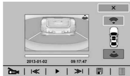
**To Activate :** Touch Video Recorder on the Home Page. Touch
