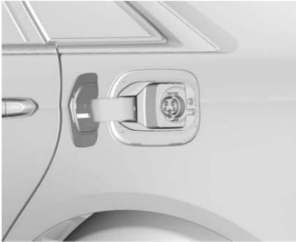
5. Plug in the vehicle plug of the charge cord into the charge port on the vehicle. Verify that the charging status indicator illuminates on top of the instrument panel and an audible beep occurs. See *Charging Status Feedback (PLUG-IN Only)* ⇨ 294.
