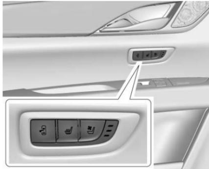
If equipped, press
