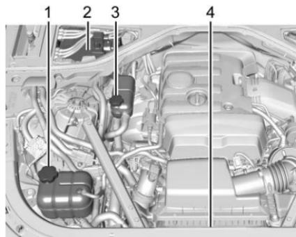
1. Engine Coolant Surge Tank and Pressure Cap
