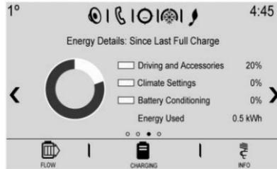
The Energy Details screen displays how energy was used since the last time the high voltage battery was fully charged. It includes Driving and Accessories, Climate Settings, and Battery Conditioning. The circle graph displays these percentages. The total energy used displays at the bottom of the screen.
