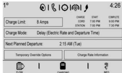
**Delay (Electric Rate and Departure Time)** : The vehicle estimates the charging start time based on the utility rate schedule, utility rate preference, and the programmed departure time for the current day of the week. The vehicle will charge during the least expensive rate periods to achieve a full battery charge by the departure time. Electrical rate information from the utility company for the charging location is required for this mode.
