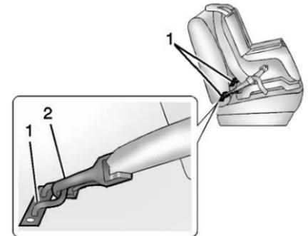
Lower anchors (1) are metal bars built into the vehicle. There are two lower anchors for each LATCH seating
