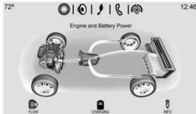
The Power Flow screens indicate the current system operating condition. The screens show the energy flow between the engine, generator, and high voltage battery. These components will be highlighted when they are active.
