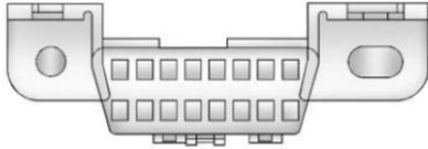
The DLC is under the instrument panel to the left of the steering wheel. Connecting devices that are not used to perform an Emissions Inspection/Maintenance test or to service the vehicle may affect vehicle operation. See *Add-On Electrical Equipment* ⇨ 315. See your dealer if assistance is needed.
