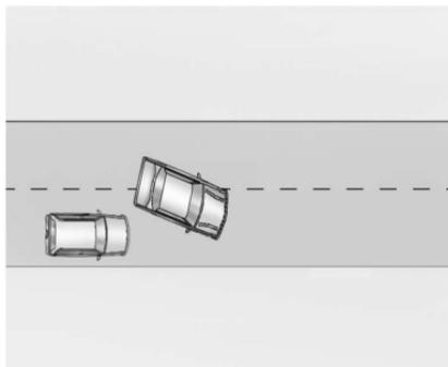
Super Cruise may not detect a vehicle that enters your lane, or brake fast enough to avoid a crash. You must manually brake and steer the vehicle.
