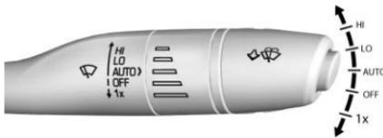
With the ignition on or in ACC/ACCESSORY, move the lever up or down to select the wiper speed.
