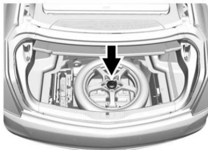
3. Turn the retainer nut counterclockwise and remove the spare tire. Place the spare tire next to the tire being changed.
