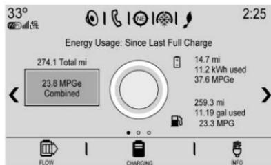
The Energy Usage screen displays information for the total of all drive cycles since the last time the high voltage battery was fully charged. This includes:
