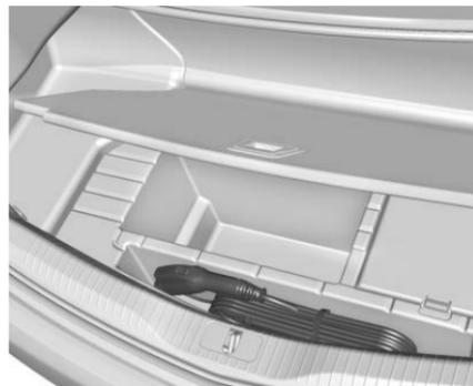
3. Open the trunk. Lift the load floor cover and remove the charge cord.
