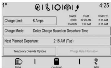
**Delay Charge Based on Departure Time** : The vehicle estimates the charging start time considering the programmed departure time for the
