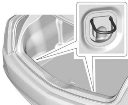
The cargo tie-downs can be used to secure small loads and the convenience net. See *Convenience Net* ⇨ 119, if equipped.
