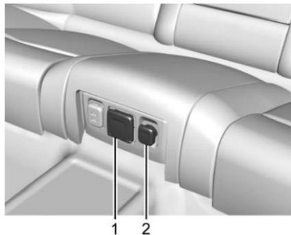
1. Power Outlet 110V/120V Alternating Current
