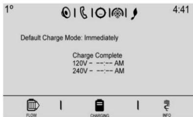
When the Programmable Charging system is disabled, the Default Charge Mode Status screen and the pop-up will display “- :-:-” for the Charge Complete Time. The Programmable Charging system will be disabled if the Charge Complete Time cannot be
