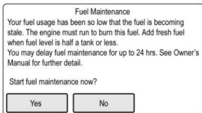
When FMM is needed, the FMM Request screen appears on the infotainment display at vehicle start.
