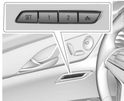
If equipped, memory seats allow two drivers to store and recall their unique seat positions for driving the vehicle, and a shared exit position for getting out of the vehicle. Other feature positions may also be set, such as power mirrors and power steering wheel. Memory positions are linked to RKE transmitter 1 or 2 for automatic memory recalls.
