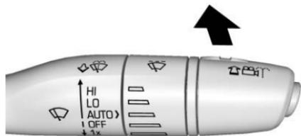
If equipped, push the windshield wiper lever forward to spray washer fluid on the rear camera lens. The lever returns to its starting position when released. See *Rear Camera Mirror* ↪ 57.
