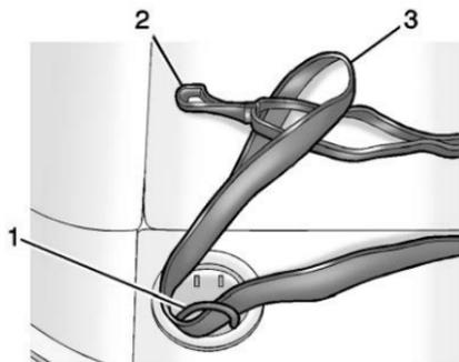
5. Route the loop end of the strap (3) through one of the cargo tie-downs (1) in the rear of the vehicle.
