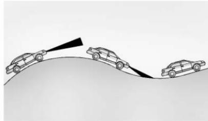
Do not use ACC when driving on steep hills or when towing a trailer. For towing capability, see *Trailer Towing (PLUG-IN Only)* ⇨ 313 or *Trailer Towing (Gasoline Only)* ⇨ 313. ACC will not detect a vehicle in the lane while driving on steep hills. The driver will often need to take over acceleration and braking on steep hills, especially when towing a trailer. If the brakes are applied, the ACC disengages.
