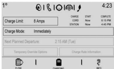
**Immediately** : The vehicle starts charging as soon as it is connected to an electrical outlet. See *Plug-In Charging (PLUG-IN Only)* ⇨ 292.
