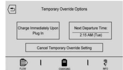
2. Touch Charge Immediately Upon Plug In to temporarily override to an Immediate Charge Mode.
