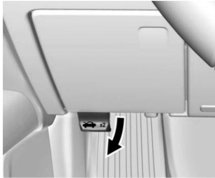
1. Pull the hood release handle. It is on the lower left side of the instrument panel between the door and the steering wheel.
