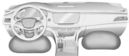
The driver knee airbag is below the steering column. The front outboard passenger knee airbag is below the glove box.
