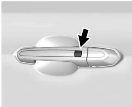
Press the lock/unlock button when the RKE transmitter is within 1 m (3 ft) of the driver door handle. When unlocking from the driver door, the first press unlocks that door; press again within five seconds to unlock all passenger doors. See *Remote Keyless Entry (RKE) System Operation* ⇨ 35.
