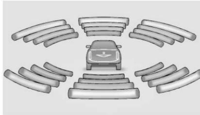
The instrument cluster may have a parking assist display with bars that show “distance to object” and object location information for the Parking Assist system. As the object gets closer, more bars light up and the bars change color from yellow to amber to red.
