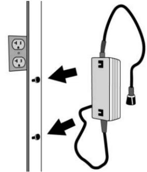
5. Securely mount the charge cord on to the screws.
