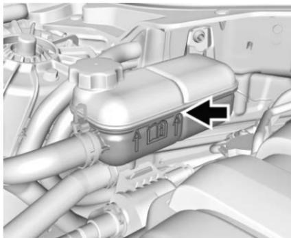
Check to see if coolant is visible in the reservoir. If coolant is visible but the coolant level is below the indicated mark, there could be a leak in the cooling system.
