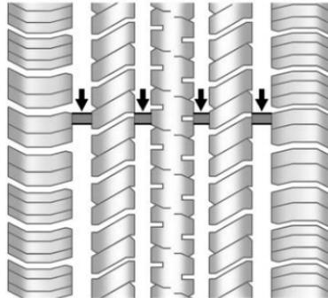
Treadwear indicators are one way to tell when it is time for new tires. Treadwear indicators appear when the tires have only 1.6 mm (1/16 in) or less of tread remaining. See *Tire Inspection* ⇨ 375 and *Tire Rotation* ⇨ 376.
