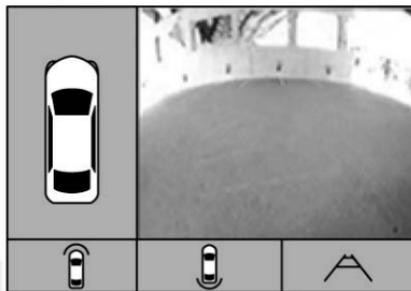
If equipped, a view of the area in front of the vehicle displays in the infotainment display. The view displays after shifting from R (Reverse) to a forward gear, or by pressing CAMERA in the center stack, and when the vehicle is moving forward slower than 8 km/h (5 mph).
