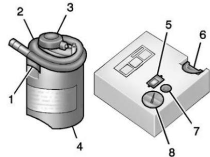
1. Sealant Canister Inlet Valve
