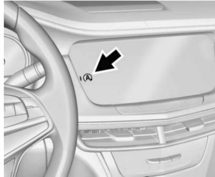
The automatic engine stop/start function can be disabled by touching (A) on the center stack.
