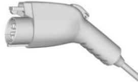
2. Unplug the vehicle plug of the charge cord from the vehicle.
