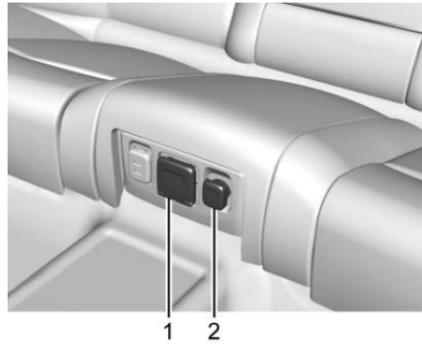
1. Power Outlet 110V/120V Alternating Current
