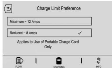
The Charge Limit Preference should be configured to match the electrical current rating for the electrical outlet that the charge cord is connected to. The Charge Limit Preference settings are:
