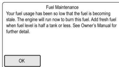
If the FMM request was delayed for one day, FMM will start at the next vehicle start and display the FMM Notification screen on the infotainment display. The engine will not start until after a short delay once shifted into D (Drive).
