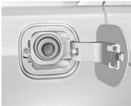
To open the fuel door, push and release the rearward center edge of the door. If equipped, the fuel door is locked when the vehicle doors are locked. Press
