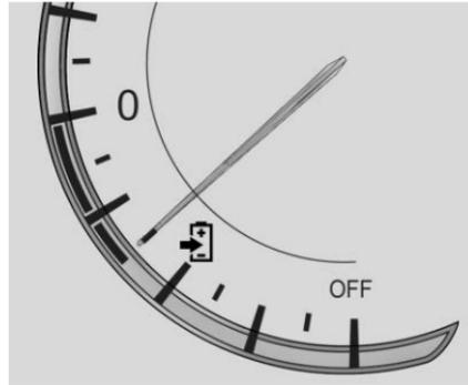
The power gauge shows the vehicle's total power consumption coming from the engine and/or battery.
