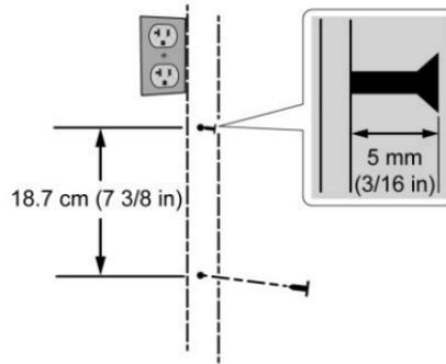
3. Mark and drill the mounting holes in a wall stud or suitable structure. Stay away from any power source.
