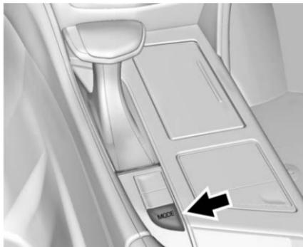
Press and release MODE to activate the mode menu in the instrument cluster. The first press of the button will show the current mode. Subsequent presses will scroll through the available modes. Select a new setting whenever driving conditions change. The following modes are available:
