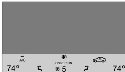
The climate control status display appears briefly when the climate control buttons on the center stack are adjusted.
