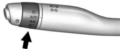
The exterior lamp control is on the turn signal lever.
