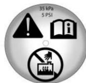
The coolant reservoir pressure cap can be removed when the cooling system, including the pressure cap, is no longer hot.
