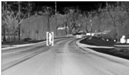
With the Front Pedestrian Braking system turned on, Night Vision provides a red Head-Up Display (HUD) alert when the system detects that the vehicle is approaching a pedestrian ahead much too quickly. In addition, an alert beeps or the Safety Alert Seat pulses, if equipped. See *Front Pedestrian Braking (FPB) System* ⇨ 281.
