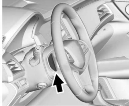
2. Tap the left control on the back of the steering wheel toward the driver to select more coast deceleration. Tap the right control toward the driver to select less coast deceleration. To select the most coast deceleration, press and hold the left control.
