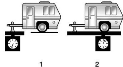
In general, trailer tongue weight (1) should be 10% of the loaded trailer weight (2). Some specific trailer types, such as boat trailers, fall outside of this range. Refer to the trailer owner's manual for the recommended trailer
