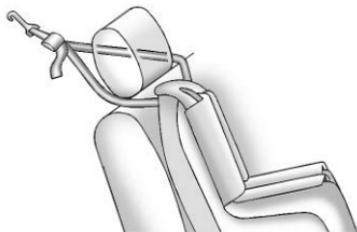
If the position you are using has an adjustable headrest or head restraint and you are using a dual tether, fully raise the head restraint and route the tethers around the outboard side of the Head Restraint posts.
