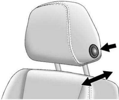
The fore and aft position of the head restraint can be adjusted.
