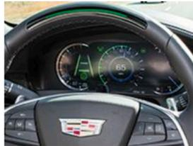
Super Cruise uses a camera to watch where the driver's eyes are looking.
